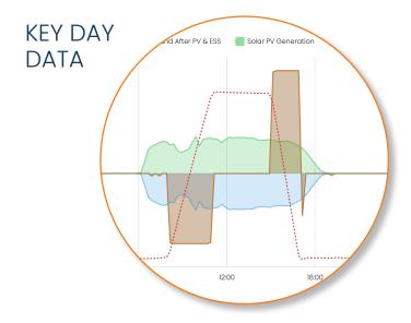
OECC pays a demand charge to a larger electric generation and distribution cooperative. To reduce its systemwide peak, OECC uses ETB Controller to strategically dispatch front-of-the-meter ESS assets, as shown in the monthly data (below). The key day data (above) show a typical utility-controlled dispatch, which effectively shifts off-peak solar generation in time to offset the late-afternoon peak demand.
