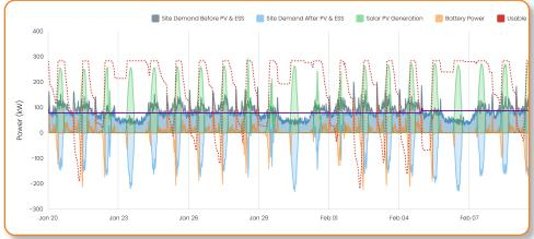
During the workweek, the beverage distribution warehouse facility experiences multiple daily load spikes, as shown in the monthly data (left). While solar production is coincident with some load spikes, as shown in the daily data (above), others occur in the early morning or evening hours. ETB Controller with Acumen AI dispatches as needed to shave the peak and maintain the demand set-point threshold.
