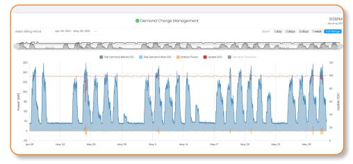
The monthly data (left) for the American Faucet factory are punctuated by relatively narrow and extreme peaks. While the ESS capacity is just 7.6% of the peak load, ETB Controller with Acumen AI is highly successful at dispatching stored energy to offset NC demand. The daily data (above) shows the maximum NC demand with and without ESS. On this key day, the 29.4 kW–rated battery shaved the midday peak demand by 28 kW.
